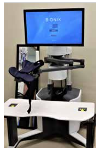
The Bionik Arm provides a way for patients to retrain their muscles to refine their movements through observation and repetition.
